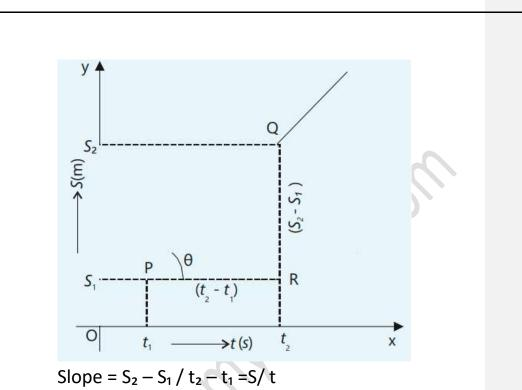
S = v , the average speed during the time interval t. Now S/t = tan  $\theta$  = slope of graph line.
