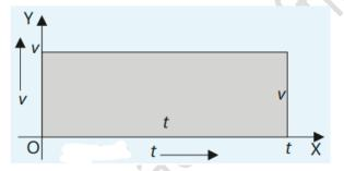
This distance can also be found by calculating the area under the speed-time graph. The area under the graph for time interval t is the area of rectangle of sides t and v. This area is shown shaded in Fig.2.23 and is equal to  $v \times t$ . Thus, area under speed-time graph up to the time axis is numerically equal to the distance covered by the object in time t.
